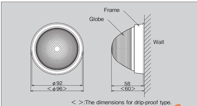
The location lamp has a high luminance with which the light from the lamp can be clearly visible at a position 10m apart from the location lamp along with a direction of an angle of 15° or more from the mounting surface.
