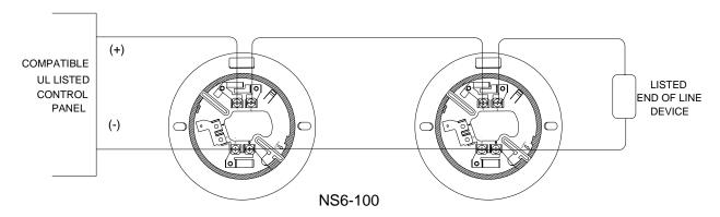
Non polarized, not current limited. No annunciator output.
